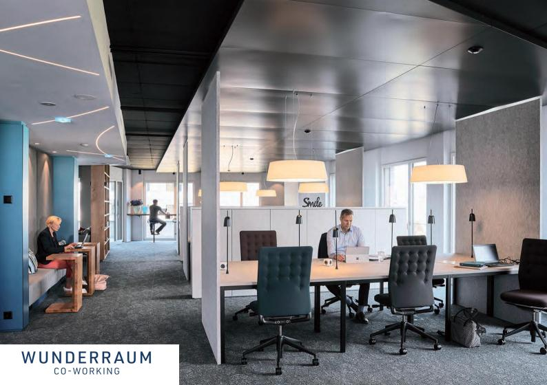
Wunderraum co-working space provide different work settings that requires different acoustic treatments. Acoustic wall claddings are widely used in shared and open spaces and acoustic dividers are installed in focus areas.
